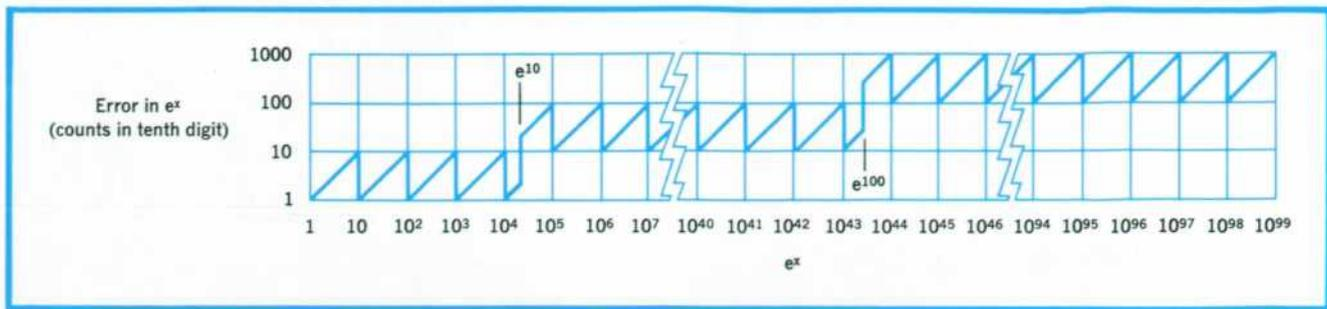
**Fig. 1.** Accuracy of exponential function in HP-35 Calculator. Error bound is approximately  $\delta e^x$ , where  $\delta$  is the error due to prescaling and the algorithm itself.  $\delta$  is estimated to be equivalent to one count in the tenth significant digit of the argument  $x$ .
