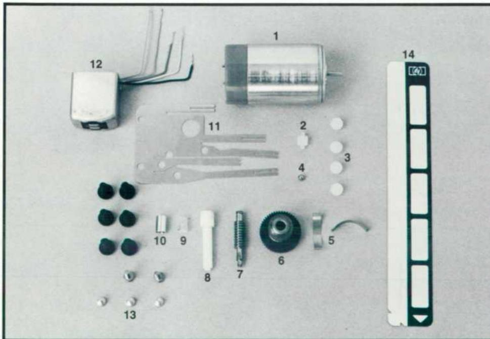
**Fig. 2.** HP-65 card reader parts: 1. Motor 2. Idler roller 3. Switch activation balls 4. Thrust ball bearing 5. Card side loading springs 6. Rubber drive roller and helical gear 7. Worm gear 8. Drive pin 9. Coupler 10. Coupler sleeve 11. Switch contacts 12. Read/write head 13. Self-tapping switch adjustment screws 14. Magnetic card, 7.1 cm by 1 cm.
