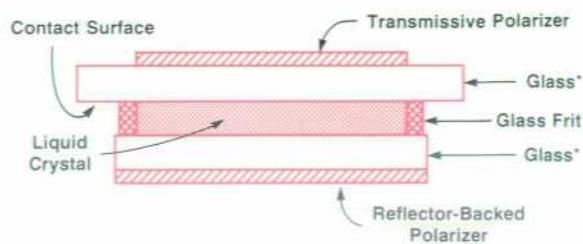
\*Inside surfaces of glass coated with a patterned, transparent layer of indium and tin oxides.
