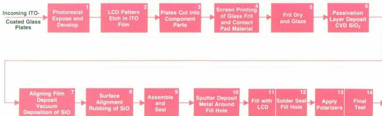
**Fig. 4.** HP-41C liquid crystal display manufacturing process.
