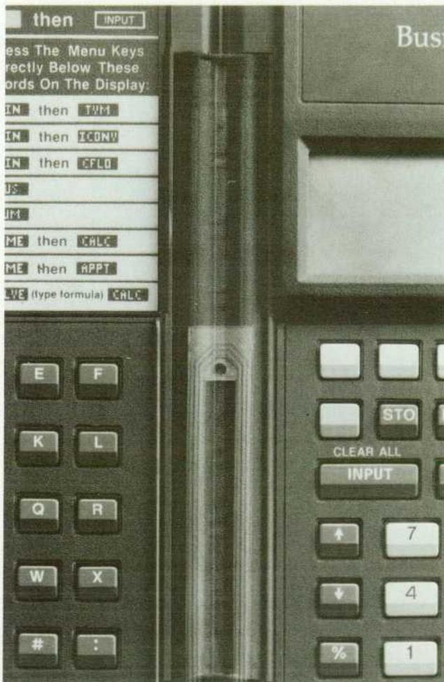
Fig. 3. Double exposure photograph showing shape of flex circuit and its location within the hinge assembly.
