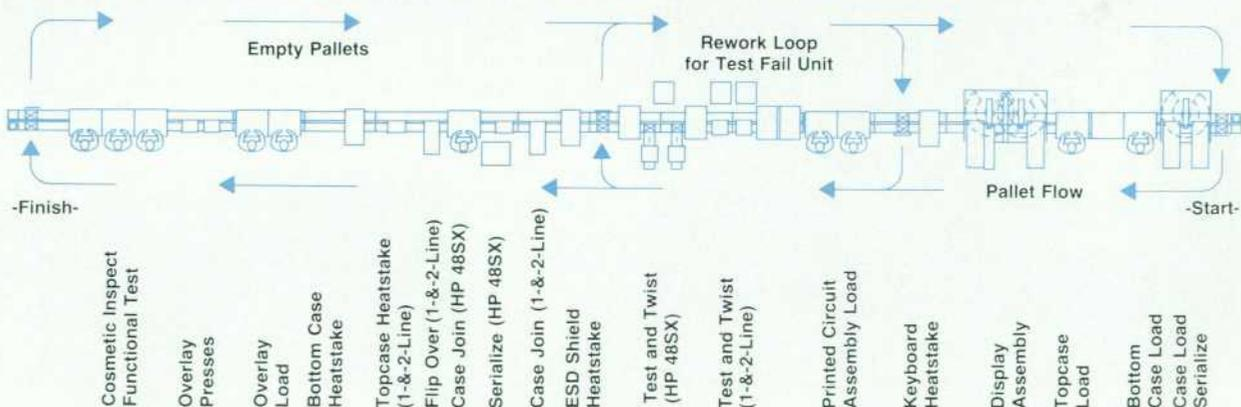
Fig. 4. HP 48SX final assembly line layout.
